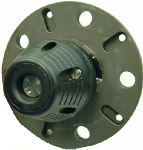
The Drive Plate Torque System uses a low power radio link to transfer digitised strain measurements from a rotating wheel hub to a stationary antenna mounted nearby. The signals are passed to a receiver where they are decoded and output as CAN bus messages and analogue outputs.
